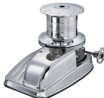
DK6 DY Passacatena sinistro con campana Left chain pipe with drum
