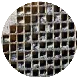
PARTIALLY BLOCKED DPF
